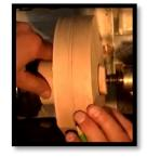
From experience he wants the sides to narrow to approximately 1/4". Accordingly, after marking the centre line, he adds two lines on either side that are 1/8" from the centre.
