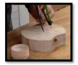
To centre the glue block on the turning, he sets a compass approximately 1/16" greater than the diameter of the block and transfers this dimension to the turning. As a transparent adhesive is necessary to see the pencil line, Gord uses thick CA glue which also provides a bit more working time.
