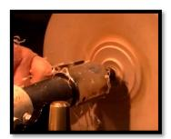
Once completed he re-engages the tailstock using the "button" to protect the face of the turning. As he did with the first side, he completes this face using a high-sheer pull cut. However, he finds that at the outer edges this produces a considerable amount of tear out. Accordingly, he sands each side by hand to bring it to the desired mark.
