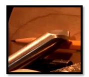
He starts on the outside edge of the face where he will need to remove a considerable amount of wood. While he initially takes a relatively robust cut — which produces a considerable amount of tear out — as he gets closer to the final mark, he adopts a lighter cut for a smoother finish.
