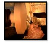
He removes the tailstock to complete turning the face. He begins in the centre to remove the compass point before faring this area into the balance of the face. Once again, he sharpens the tool before making the final cuts.
