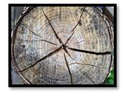
Hence, the primary goal in drying wood is to attempt to ensure a relatively equal moisture content and thus drying time throughout a blank. For example, in the case of commercial kilndried wood, heat and steam are introduced into the drying chamber at scheduled times to maintain a moisture level on the outside of the wood the same as that on the inside.
