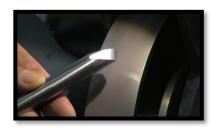
For most of his turning, Tim uses a bowl gouge with a swept-back grind where the wings of the tool are swept back 1-2 times the diameter of the tool.
