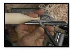
As he proceeds with the turning, he emphasized that to the extent possible, you should apply pressure towards the headstock. Applying side pressure – perpendicular to the blank may lead to a break.
