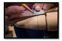
For those new to finial turning, most sources recommend drawing a proportioned sketch on graph paper in advance. This allows one to easily play with different forms and dimensions before putting tool to wood. As Cindy Drozda notes, it also means that one is not faced with the often-impossible task of making changes to a completed portion of the finial.
