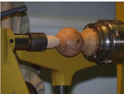
Resist the temptation to sand at this point – the sandpaper will remove end grain much less quickly than elsewhere, and the resulting shape may not hold securely enough in the chuck for the rest of the operations.
