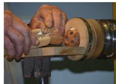
Now it's time to bring out another special tool, looking rather like an allen key with a sturdy, curved depth stop attached to its long leg. The short leg of this tool terminates in a cutting edge. Resting the tool on the platform described above, with the elbow
