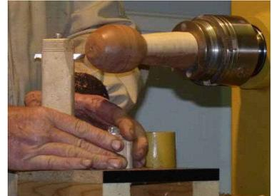
In the past we have seen a variety of ways of turning spheres using only a lathe, chisel, and scraper, but use of the special tool is recommended in this case since the rest of the process requires that the ball be perfectly spherical and of a specific size.
