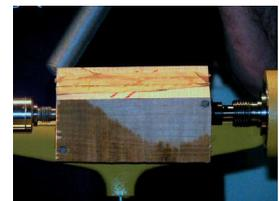
He starts the process using a roughing spindle gouge. To achieve consistent thickness without having to use calipers, Art drills small holes into the waste wood sandwiched between the two maple blanks creating a visual reference. He can now observe the thickness by simply stopping
