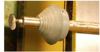
removed from the lathe and split with a wood chisel. Re-glue the goblet and remount it on the lathe. The goblet is held by a homemade tool used for his hollow forms. He now returns the goblet. Some hand sanding is required to smooth out the details. Once this is completed he applies a finish. The result is an oval goblet with a round stem.
